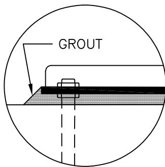
DOUBLE NUT EACH ANCHOR BOLT (LEVEL PLATE AND FILL SPACE WITH GROUT. PROVIDE 1/2-INCH DIAMETER DRAIN HOLE.)
