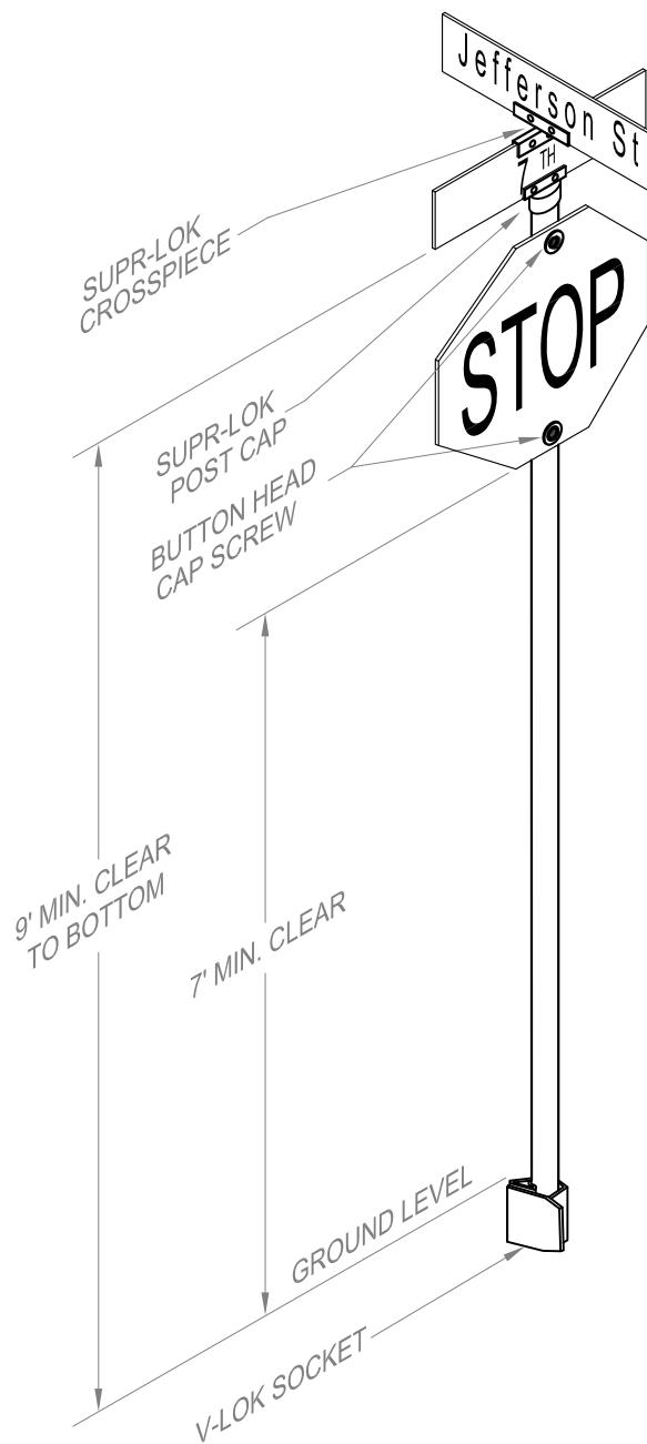
NOTE: V-LOK WEDGE SHALL FACE DIRECTION OF TRAVEL.
