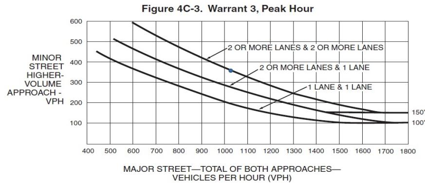
\*Note: 150 vph applies as the lower threshold volume for a minor-street approach with two or more lanes and 100 vph applies as the lower threshold volume for a minor-street approach with one lane.
