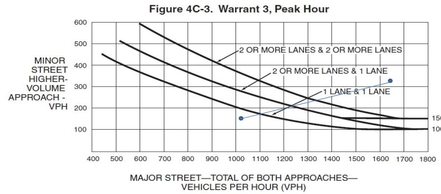
\*Note: 150 vph applies as the lower threshold volume for a minor-street approach with two or more lanes and 100 vph applies as the lower threshold volume for a minor-street approach with one lane.
