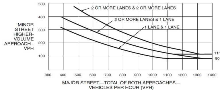
\*Note: 115 vph applies as the lower threshold volume for a minor-street approach with two or more lanes and 80 vph applies as the lower threshold volume for a minor-street approach with one lane.
